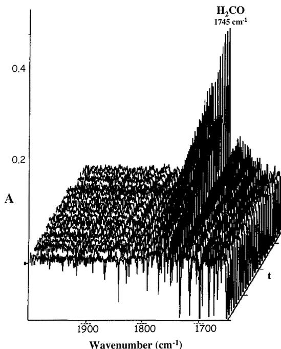
Fig. 3. Formaldehyde appearance in the simulation chamber during UV irradiation of POM. The graph present evolution of the  $\text{H}_2\text{CO}$  signature intensity at  $1745 \text{ cm}^{-1}$  as a function of time.
