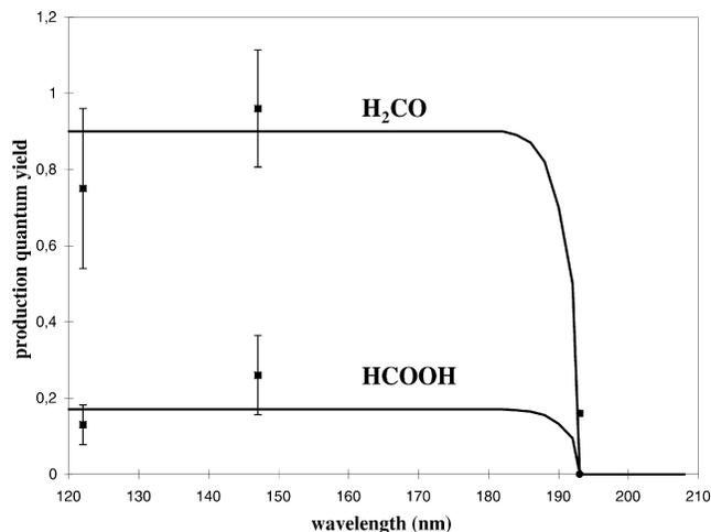
Fig. 8. Quantum yield profiles as a function of the wavelength for H<sub>2</sub>CO and HCOOH according to our experimental measurements.
