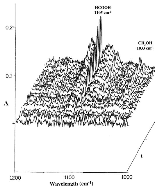
Fig. 5. Formic acid and methanol appearance in the simulation chamber during UV irradiation of POM. The graph present evolution of the HCOOH signature at  $1105\text{ cm}^{-1}$  and the  $\text{CH}_3\text{OH}$  signature at  $1033\text{ cm}^{-1}$  as a function of time.
