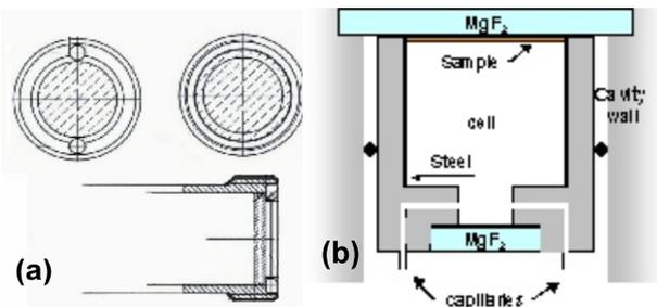
Figure 4: Cells for “AMINO” sample carrier: (a) Vented cell; (b) Close cell with an example of a sample exposed as dry film.
